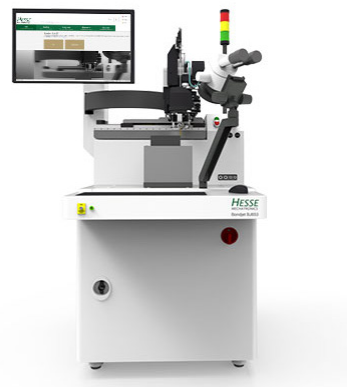
Figure 9. A fully automated wire bonding machine for high voltage production (image source: Hesse GmbH)(image source: Gpixel)
