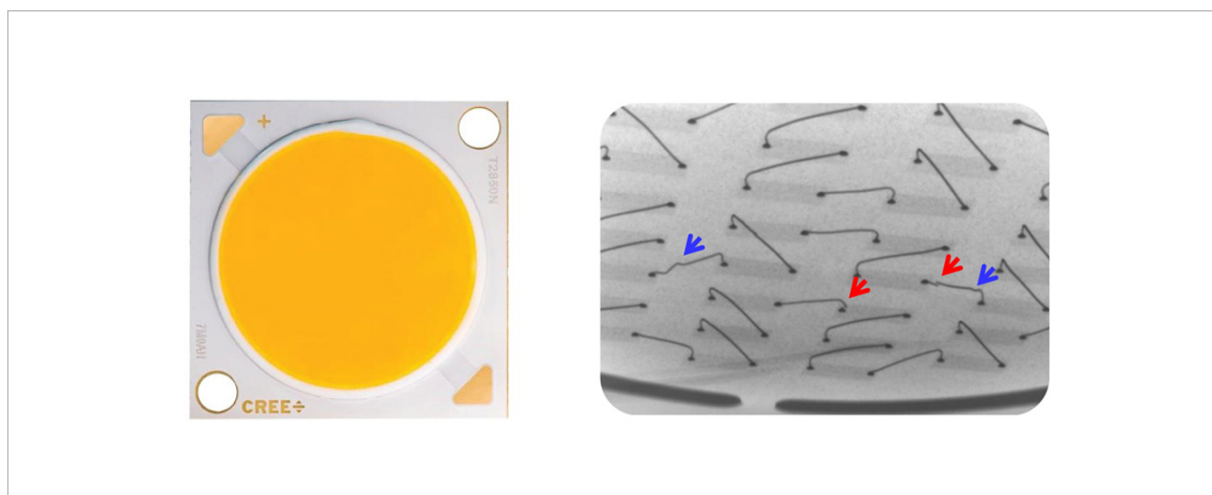
Figure 7. Example of COB LED array and x-ray image showing internal bond wires with signs of damage (image source: CREE)
