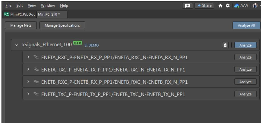
Figure 21. Net Class After Constraints Have Been Set
