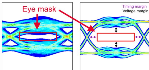
Figure 5. Left: an example of a bad eye, where the eye diagram overlaps the eye mask. Right: an example of a good eye where the eye diagram and eye mask are far apart from each other.
