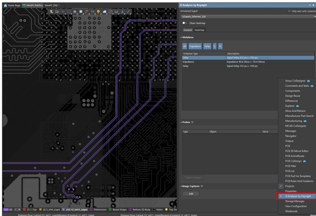
Figure 29. Where to Find the Signal Analyzer by Keysight Panel
