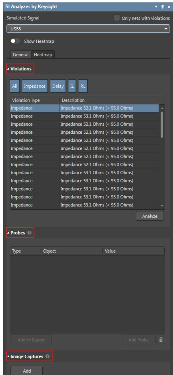
Figure 33. Sections of the Signal Analyzer by Keysight Panel
