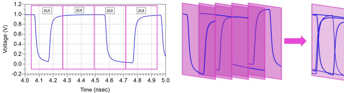
Figure 4. Top: demonstration of two-unit-interval partitions on a PRBS pattern. The eye is created after partitioning the binary sequence by every two-unit interval and stacking the partitions.
