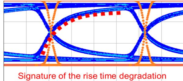
Figure 9. The signature of rise time degradation is shown in the dotted red line. Instead of a fast transition from zero to one, as in the orange eye diagram, the blue eye diagram's transitions take longer because of the frequency-dependent loss.
