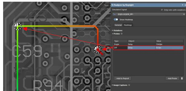
Figure 34. Probes Can Have Single Values or Take the Difference Between Two Values
