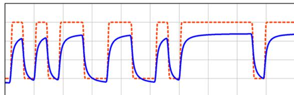
Figure 8. The loss in a channel reduces the amplitude of the signal as well as the rise time.
