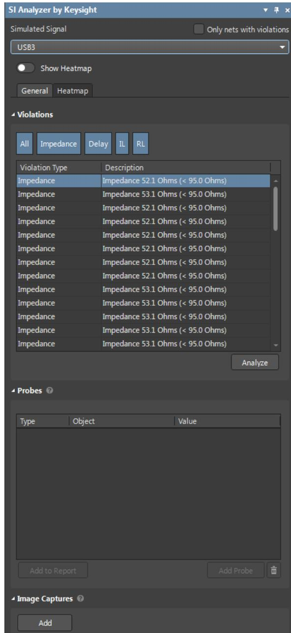
Figure 30. The Signal Analyzer by Keysight Panel
