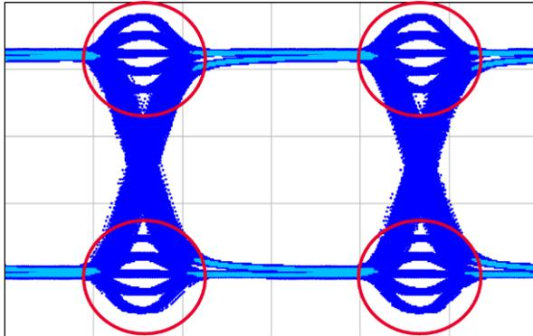
Figure 7. Typical crosstalk signature in the receiver eye looks like peaking in the transitions.
