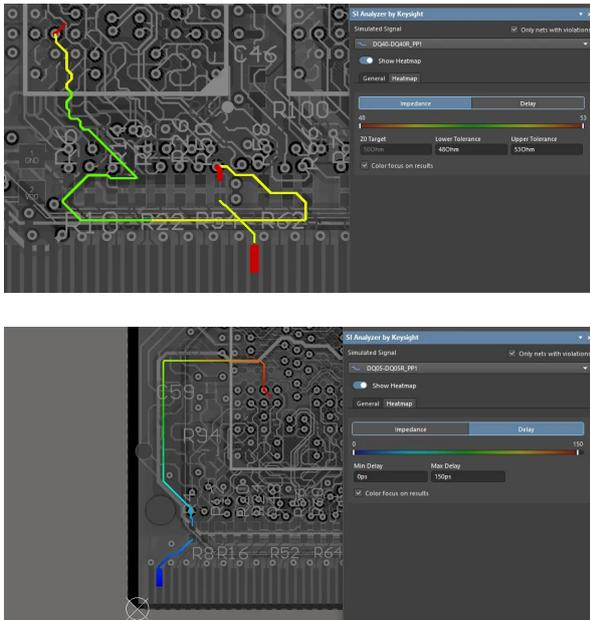
Figure 32. Select Impedance or Delay to Display the Needed Heatmap
