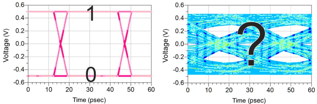
Figure 2. Left: an open eye in an eye diagram. The eye is open because a digital one or zero can be easily distinguished. Right: a closed eye in an eye diagram. The eye is closed because one cannot distinguish one from a zero.
