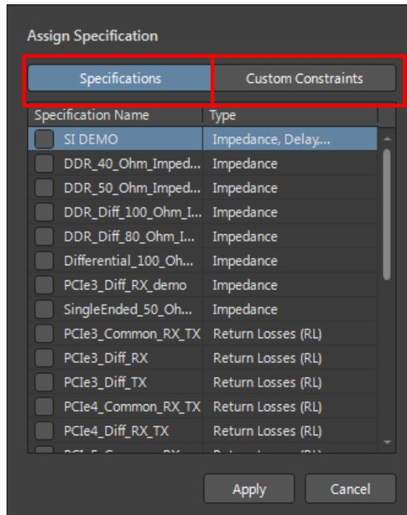
Figure 19. Select a Predefined Constraint or Create Your Own Custom Constraints
