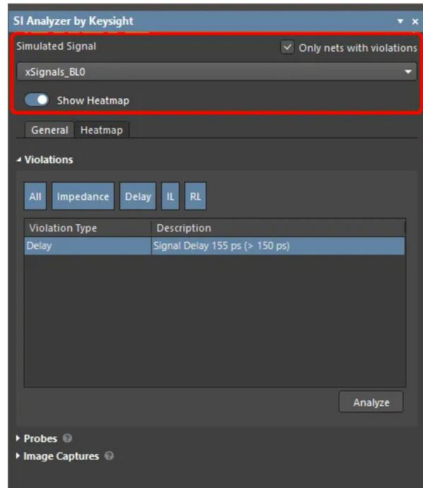
Figure 31. Choose the Signal to Analyze with the Simulated Signal Pulldown Menu
